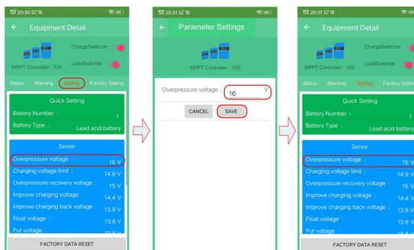
Figure 5-5 Parameter setting - overvoltage voltage setting
