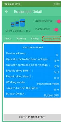
Figure 5-4 Device Details - Load Parameters
